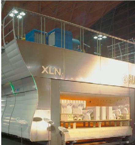
Roller hearth kiln in the ceramics industry
